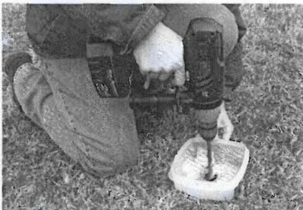
Figure 4. A power drill can facilitate sampling in rocky or dry soils. A plastic container with a hole in the middle will facilitate collecting the soil as the auger pulls it out of the ground. Empty the soil out of the plastic container into the soil sample bucket after each successful attempt to get a 6-inch core.
