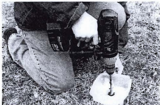
Figure 4. A power drill facilitates sampling in rocky or dry soils. Use a plastic container with a hole in the middle to collect the soil as the auger pulls it out of the ground. Empty the soil out of the plastic container into the soil sample bucket after each successful attempt to get a 6-inch core.
