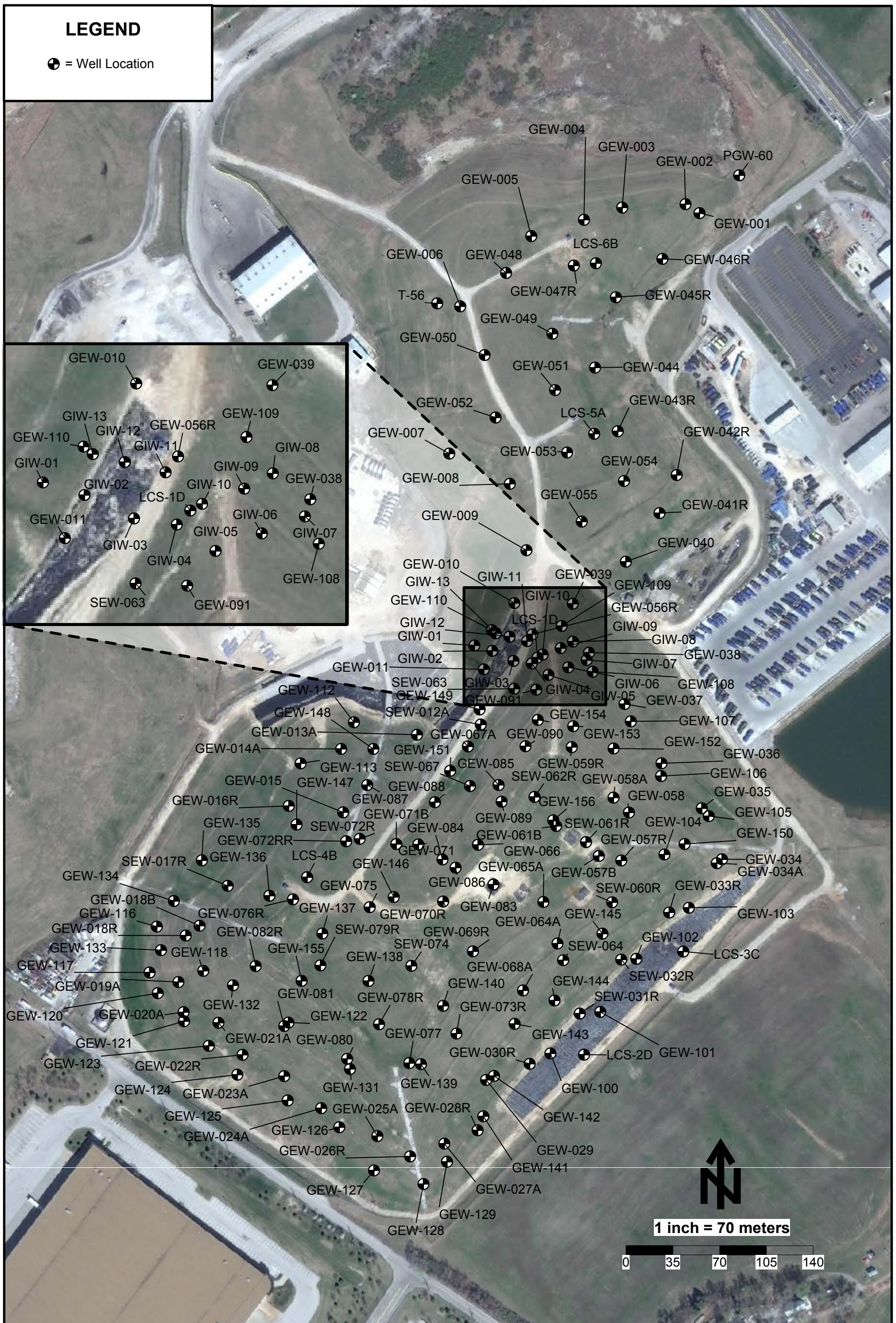
Gas Extraction Wells - Bridgeton Landfill
