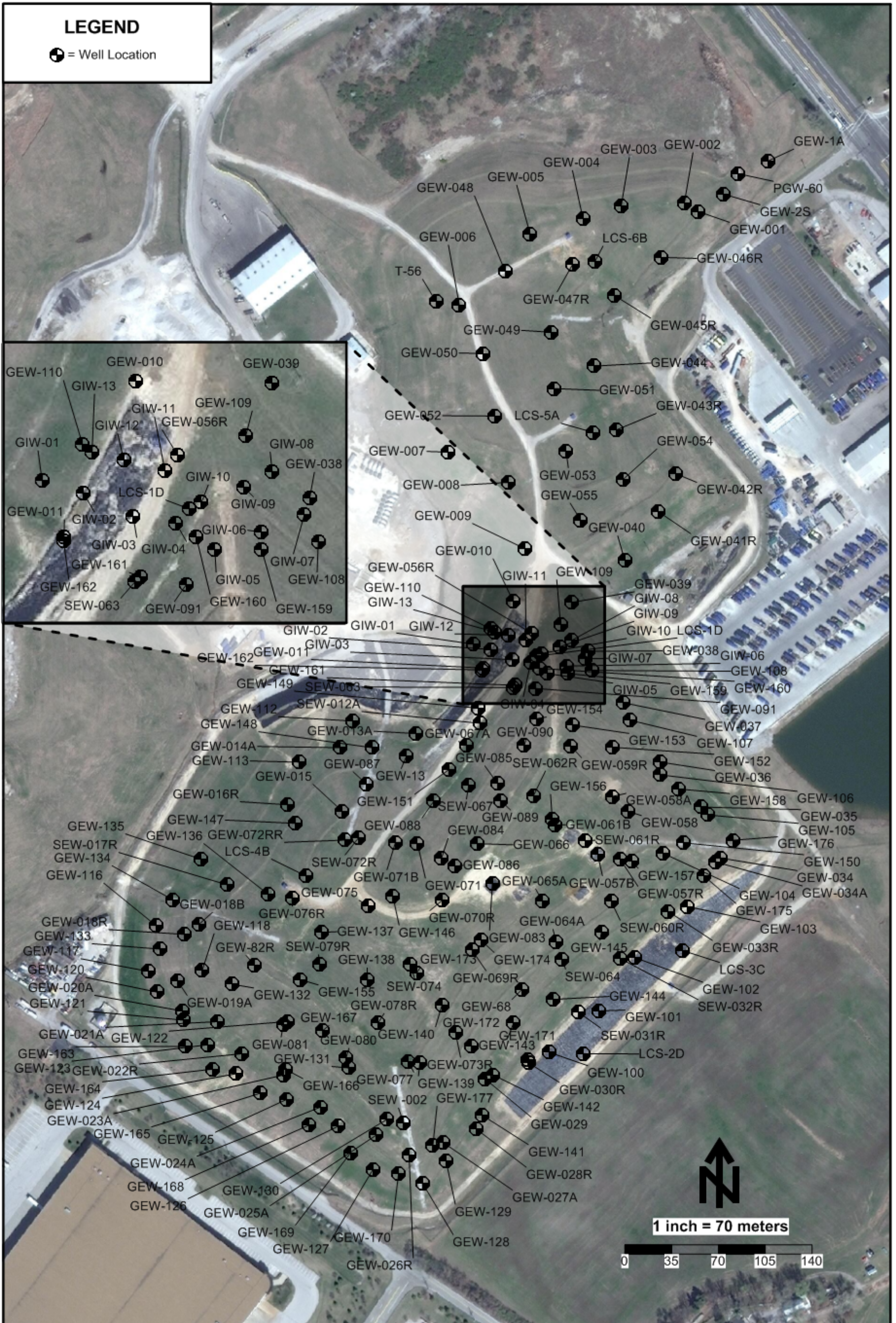
Gas Extraction Wells - Bridgeton Landfill
