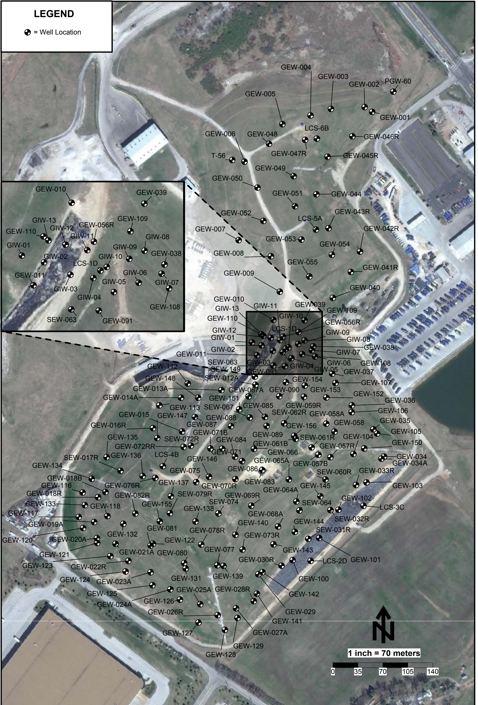
Gas Extraction Wells - Bridgeton Landfill
