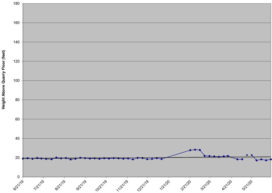
The transducer became non-operational on 1/13/20. Liquid level was measured manually on 2/21/20, 2/28/20 and 3/6/20. The transducer became operational on 3/13/20. The VFD was observed to be non-operational on 4/23/20, it was replaced on 4/23/20, however the level sensor reading was not taken due to VFD communication loss with SCADA.
