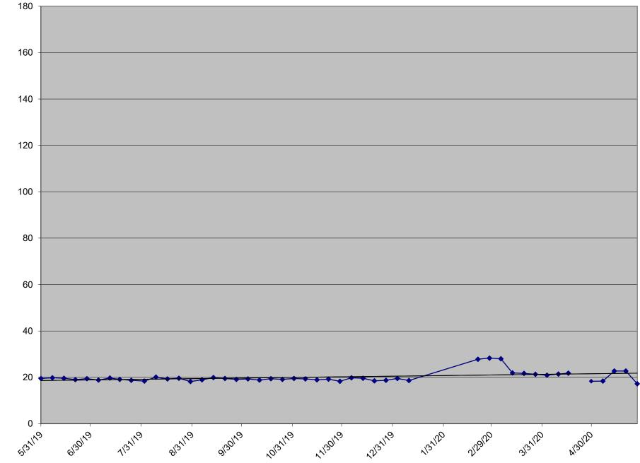
The transducer became non-operational on 1/13/20. Liquid level was measured manually on 2/21/20, 2/28/20 and 3/6/20. The transducer became operational on 3/13/20. The VFD was observed to be non-operational on 4/23/20, it was replaced on 4/23/20, however the level sensor reading was not taken due to VFD communication loss with SCADA.
