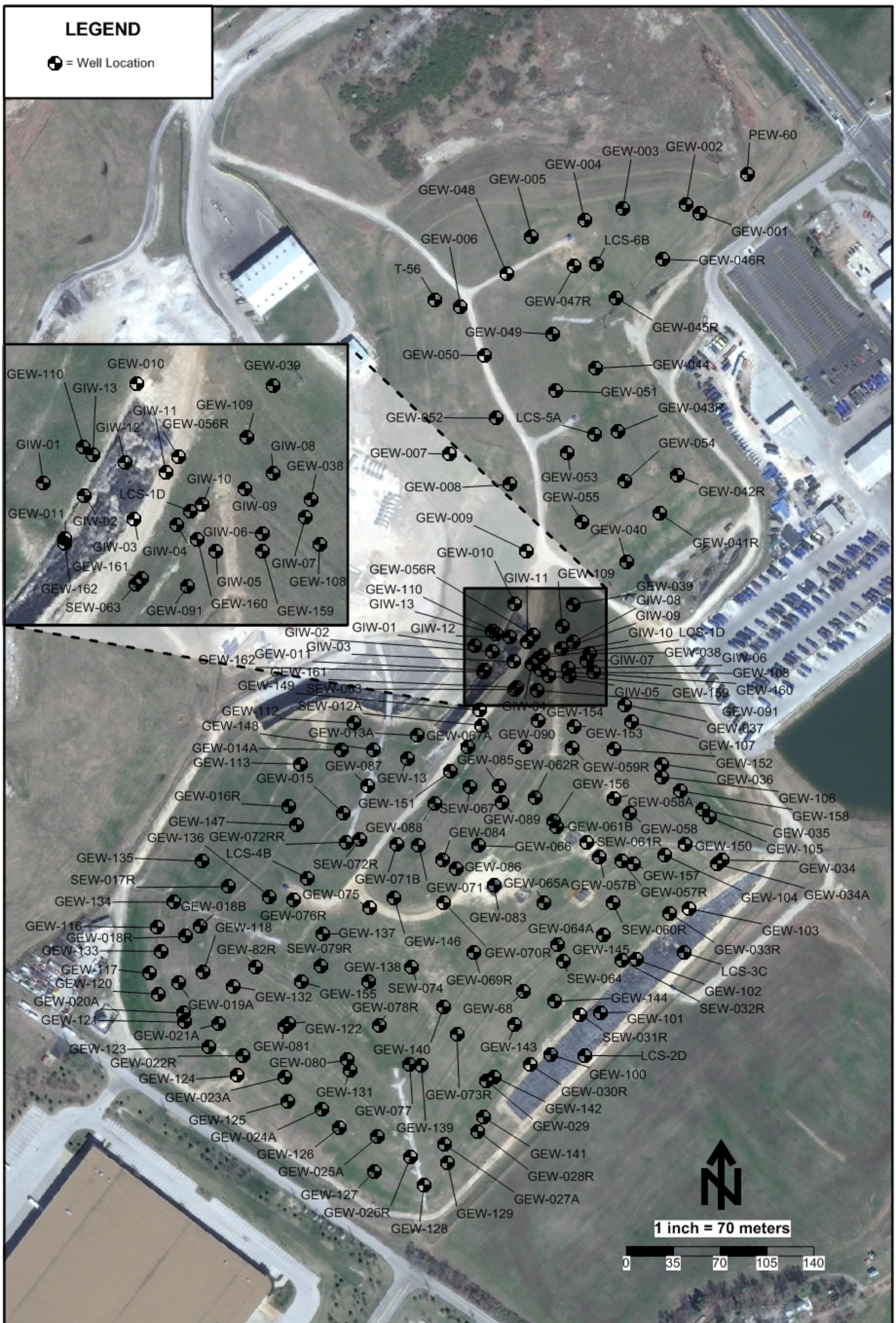
Gas Extraction Wells - Bridgeton Landfill
