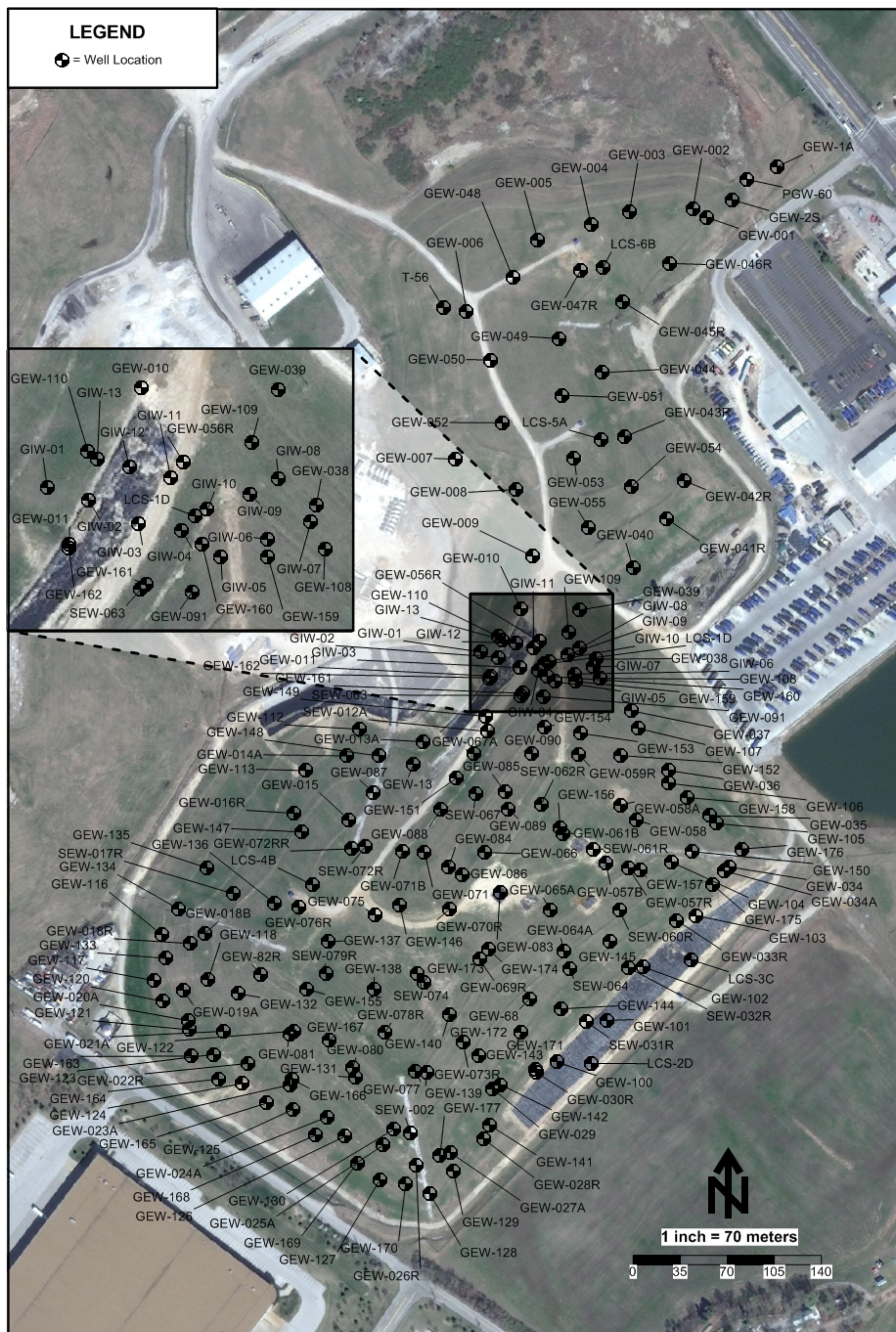
Gas Extraction Wells - Bridgeton Landfill
