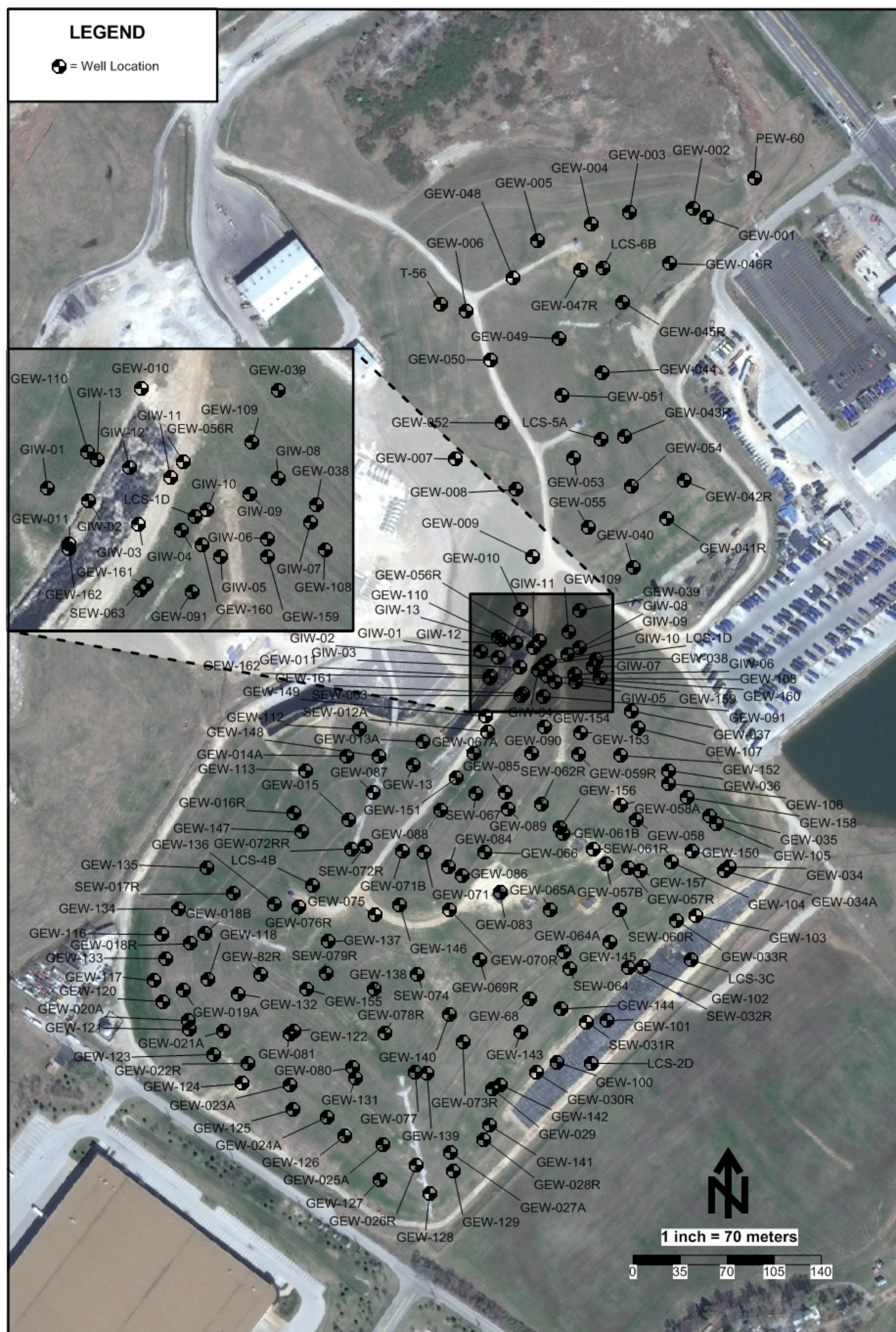
Gas Extraction Wells - Bridgeton Landfill
