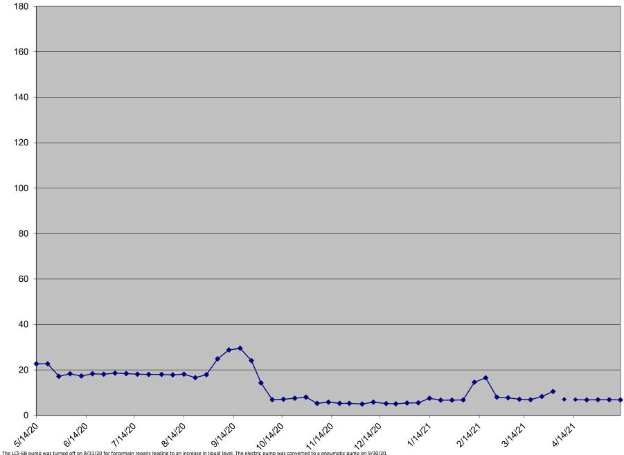
The LCS-6B pump was turned off on 8/31/20 for forcemain repairs leading to an increase in liquid level. The electric pump was converted to a pneumatic pump on 9/30/20.
