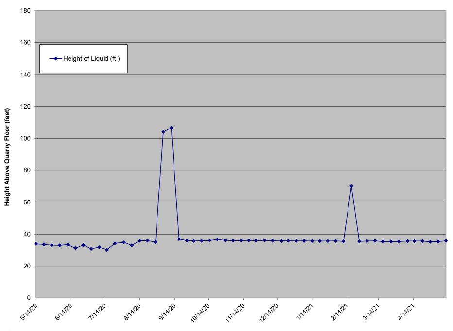
LCS-5B Liquid Level Above Quarry Floor
