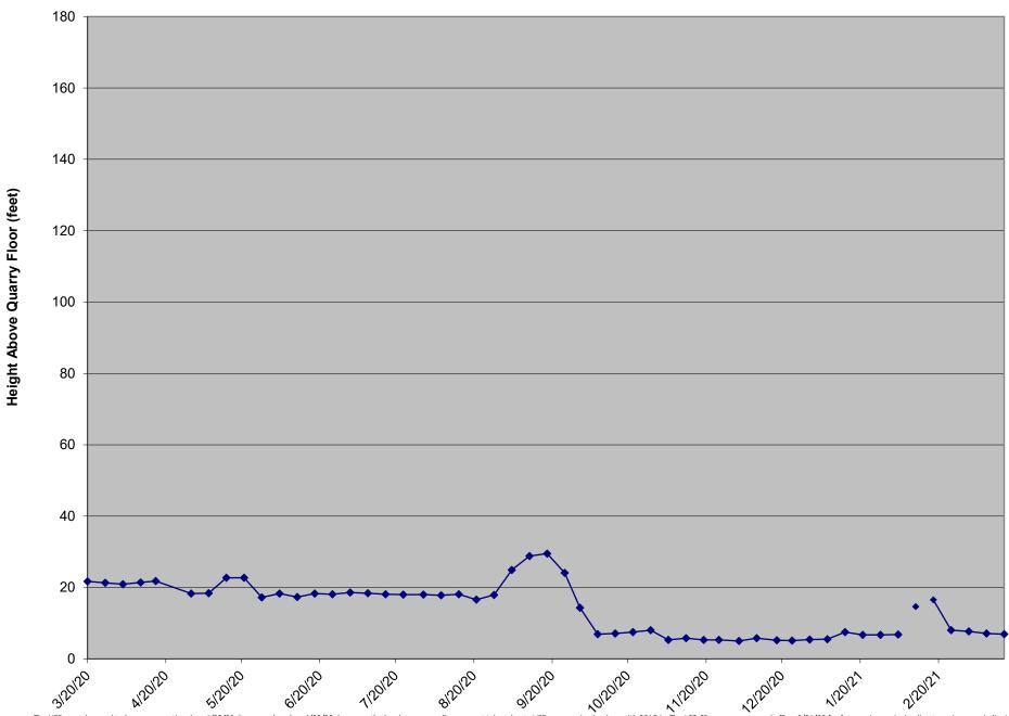
The VFD was observed to be non-operational on 4/23/20, it was replaced on 4/23/20, however the level sensor reading was not taken due to VFD communication loss with SCADA. The LCS-6B pump was turned off on 8/31/20 for forcemain repairs leading to an increase in liquid level. The electric pump was converted to a pneumatic pump on 9/30/20.
