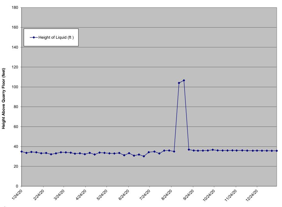
\*The LCS-5B pump was turned off on 8/31/20 for forecmain repairs leading to an increase in liquid level. The pump was replaced on 9/17/20.
