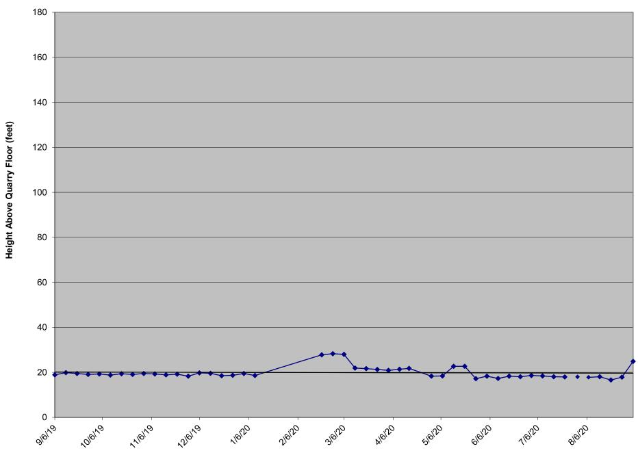
The transducer became non-operational on 1/13/20. Liquid level was measured manually on 2/21/20, 2/28/20 and 3/6/20. The transducer became operational on 3/13/20. The VFD was observed to be non-operational on 4/23/20, it was replaced on 4/23/20, however the level sensor reading was not taken due to VFD communication loss with SCADA. The LCS-6B pump was turned off on 8/31/20 for forcemain repairs leading to an increase in liquid level.
