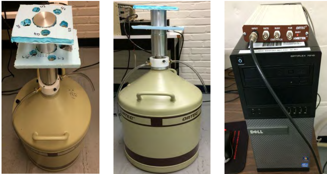
Figure 3 HPGe Detector and experimental set-up for the analysis of tree core samples for possible radioactive contamination
