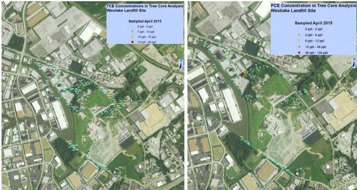
Figure 9 Mapped tree core concentrations for TCE and PCE for trees samples in April 2015 at WLL.
