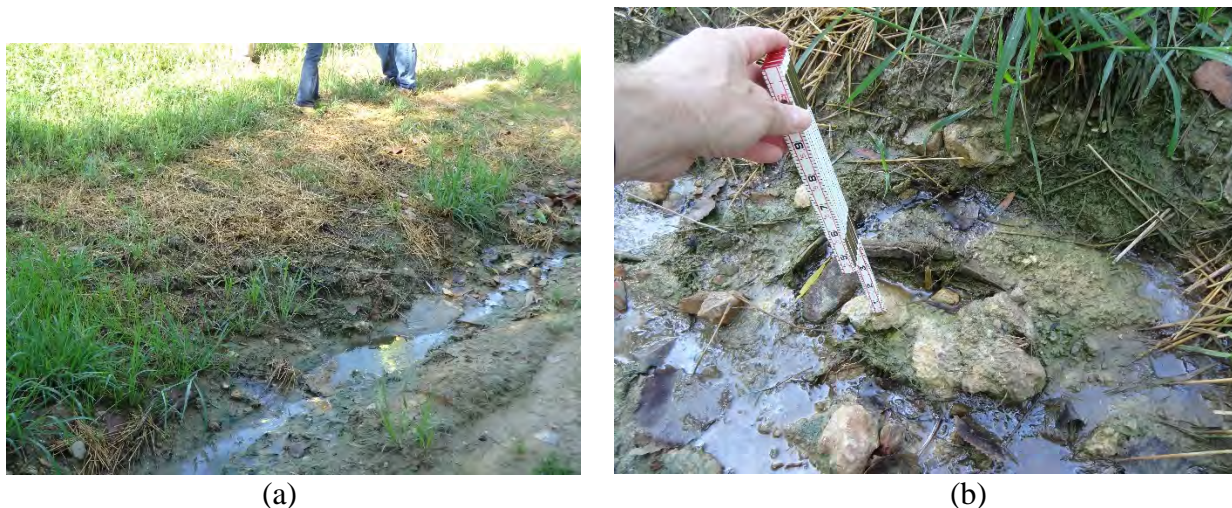
Figure 6. Photographs along north slope of north quarry showing: (a) overview of leachate outbreak and (b) close-up of leachate outbreak.
