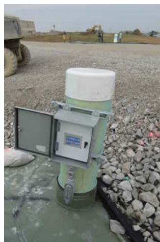
Photo of new temperature monitoring probe controllers installed in Nov. 2013 at Bridgeton Landfill.
