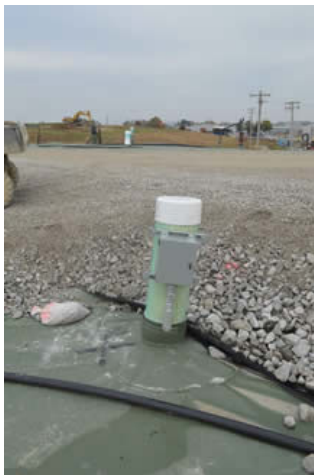
Photo of new temperature monitoring probe controllers installed in Nov. 2013 at Bridgeton Landfill.
