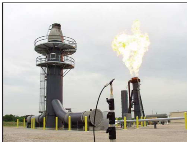
■ Figure 6. This microphone is part of the sound measurement system used for flare testing.
