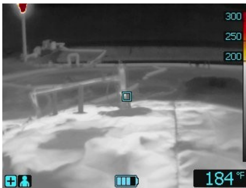
Photo 7. Thermal image of gas extraction well at Bridgeton Landfill indicating temperature of 184°F, dated April 2, 2014 (Source: Todd Thalhamer 2014)
