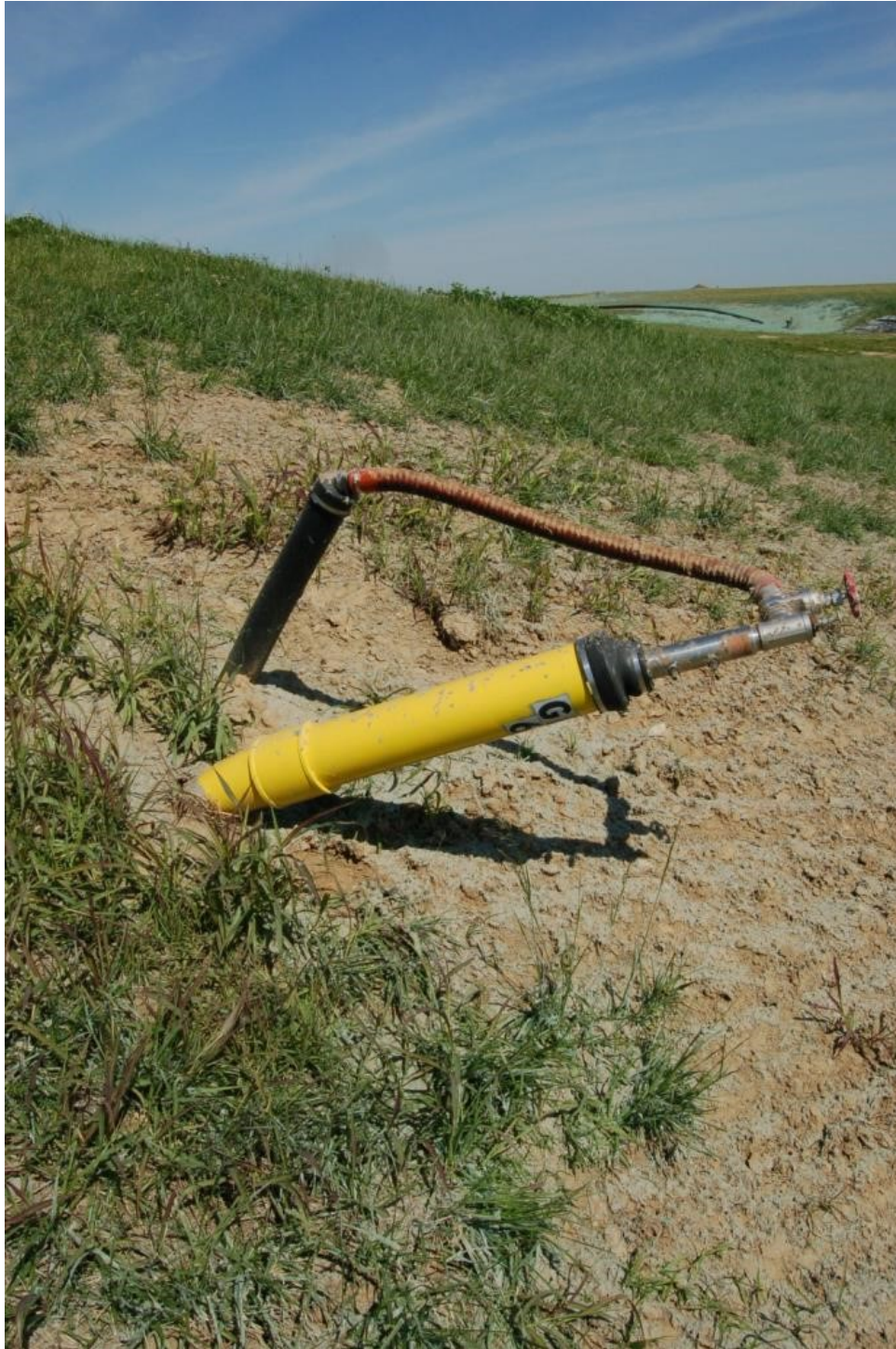
Photo 1. Damaged gas extraction well (Source: MDNR Staff 2012).
