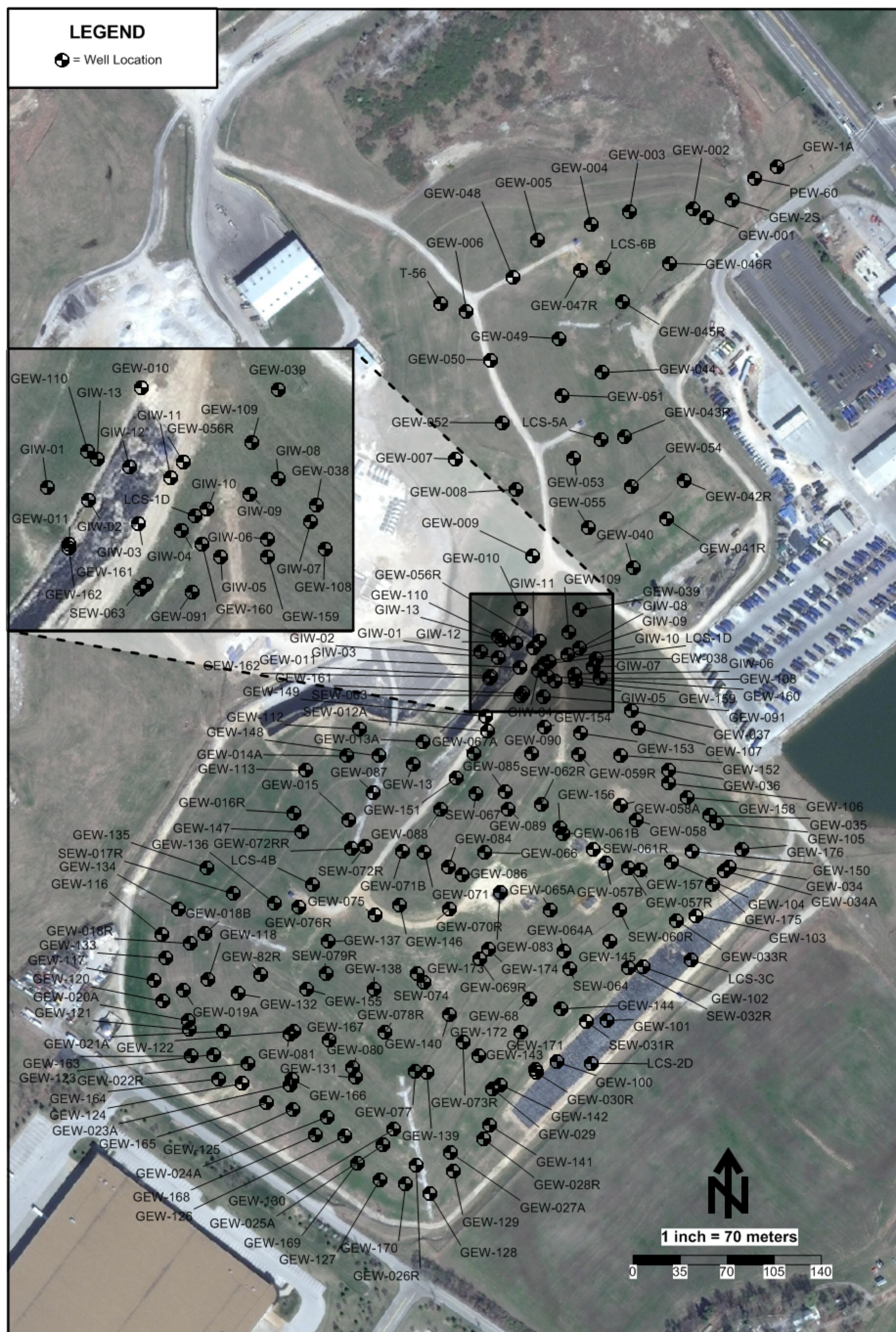
Gas Extraction Wells - Bridgeton Landfill
