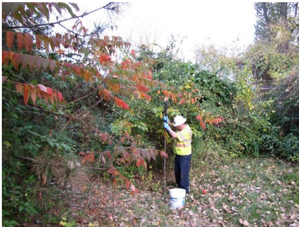
Photograph 4: Soil sampling with Split Spoon sampler
