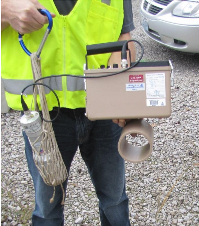
Photograph 1: EPA Ludlum 2221 with NaI 44-20 detector and directional shield attachment (EPA Equipment Y)
