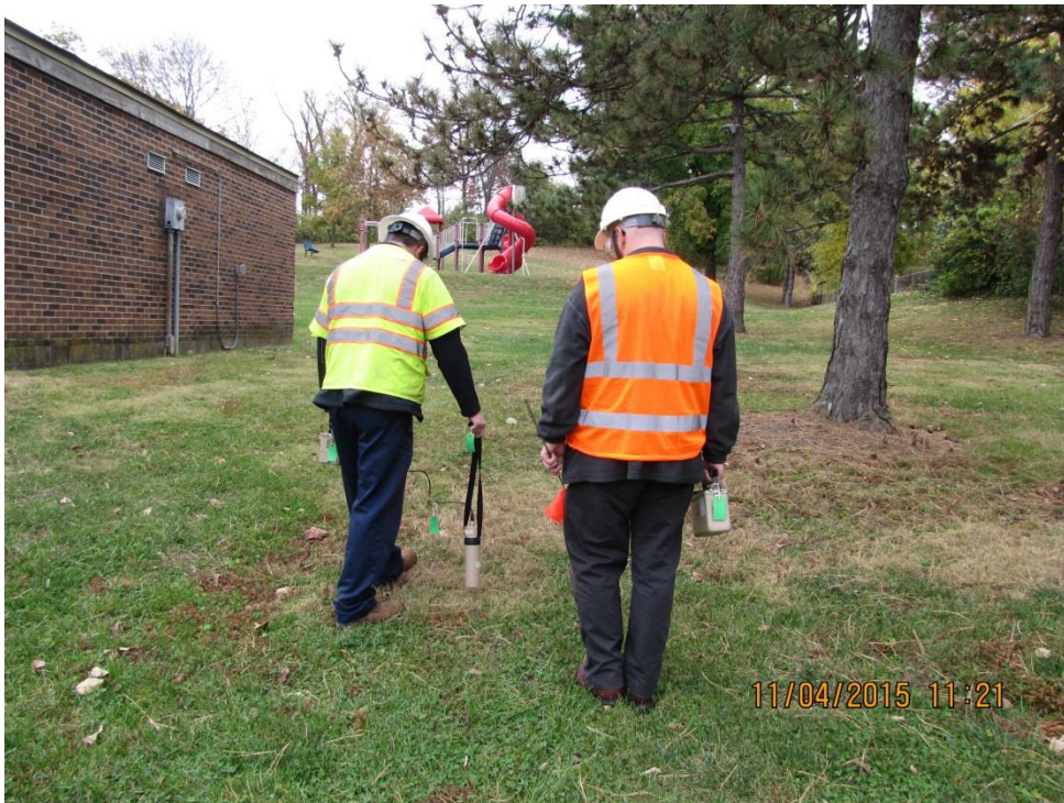
Photograph 2: Gamma walkover survey conducted at Spanish Village Park
